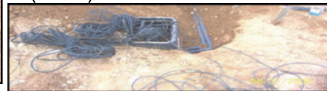
Water content reflectometer (WCR) installation
