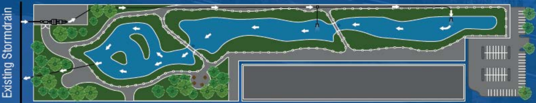
Design-phase schematic depicting water flow through the new 3-cell stormwater treatment wetland
