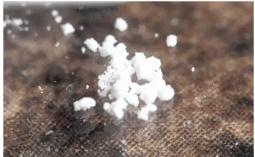
Water added to sodium polyacrylate
