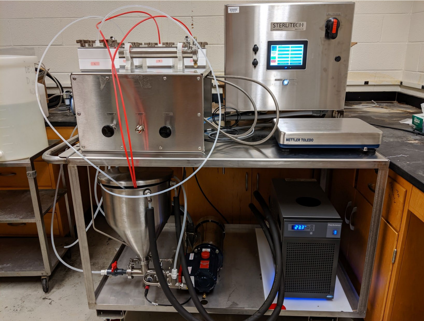
Automated cross-flow NF and Functionalized MF membranes System (4 cross flow cells, one spiral module) with temperature control, etc.)
