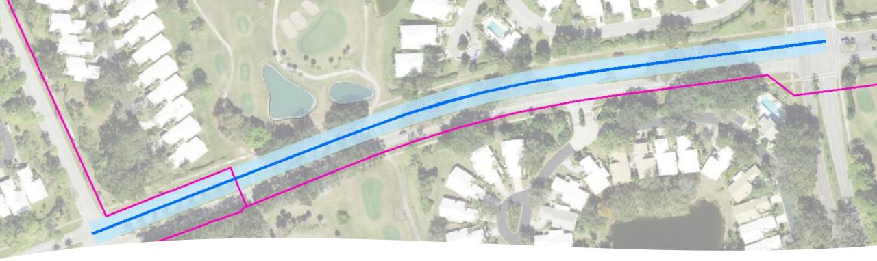
GIS used to determine conflicts impacting a route by the quantitative data involved with each 42-inch pipe segment and 50' easement
