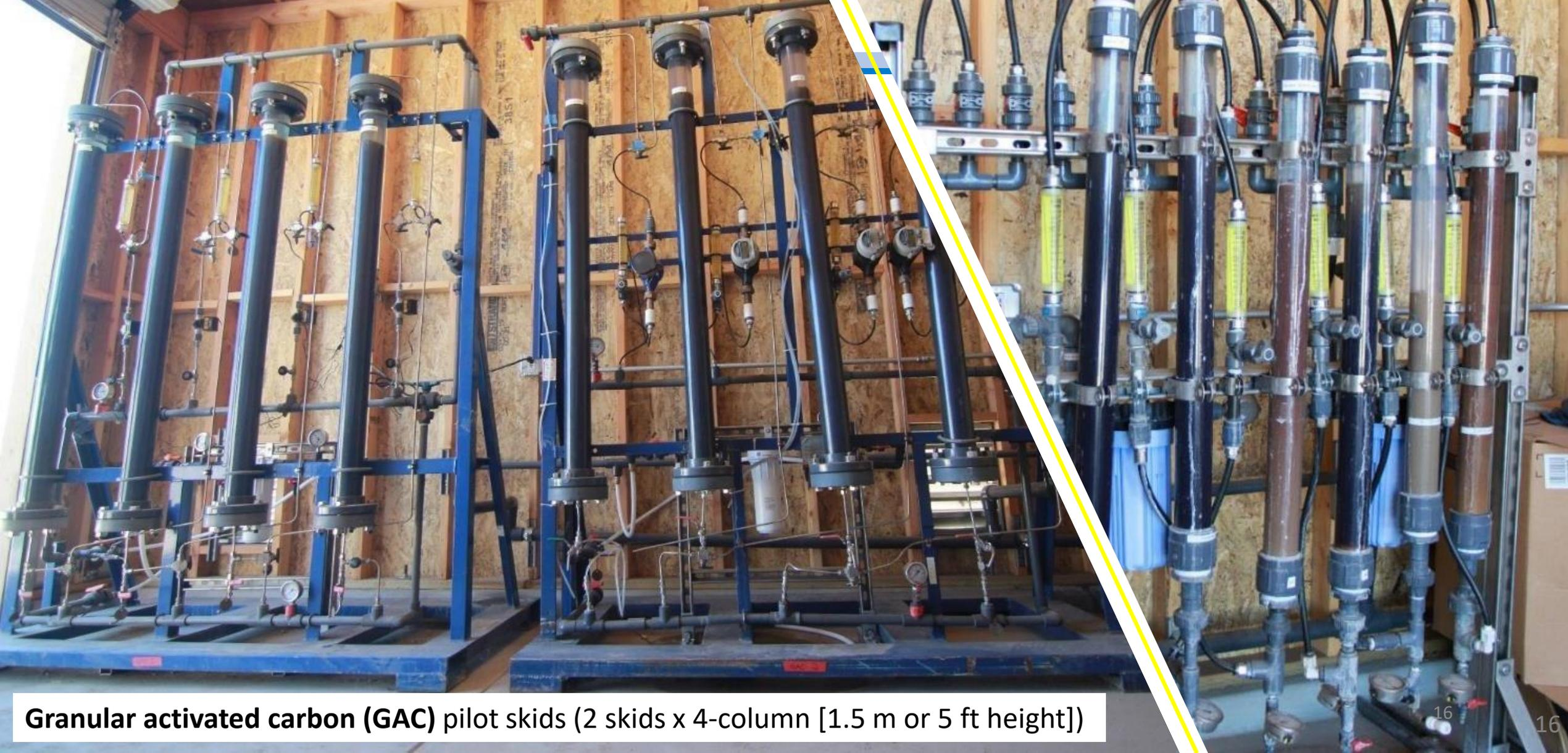
**Granular activated carbon (GAC) pilot skids (2 skids x 4-column [1.5 m or 5 ft height])**
