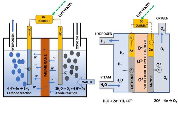
Making hydrogen and oxygen by splitting water molecule with DC current is a well-known endothermic process that uses more energy than it produces; hence it is not economical if the electricity is provided by fossil fuel power.
