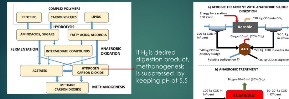
Fermentation and Methanogenesis. Products of low pH fermentation and oxidation are acetates and hydrogen that are used by methanogens to make methane in the methanogenesis step
