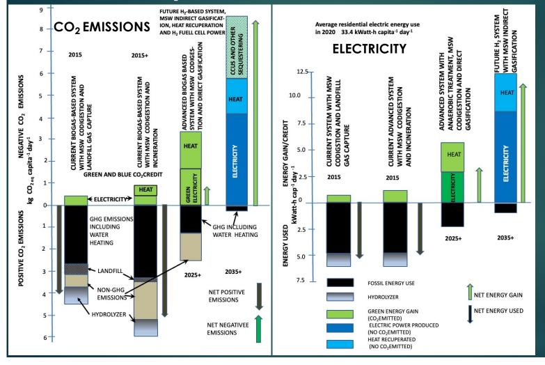
The differences between the Alternatives 1 and 2 and 3 and 4 are due to switching from landfilling of MSW, limited MSW processing by co-digestion, incineration and producing electricity by waste heat of incineration to MSW and sludge gasification and hydrogen fuel cells.
