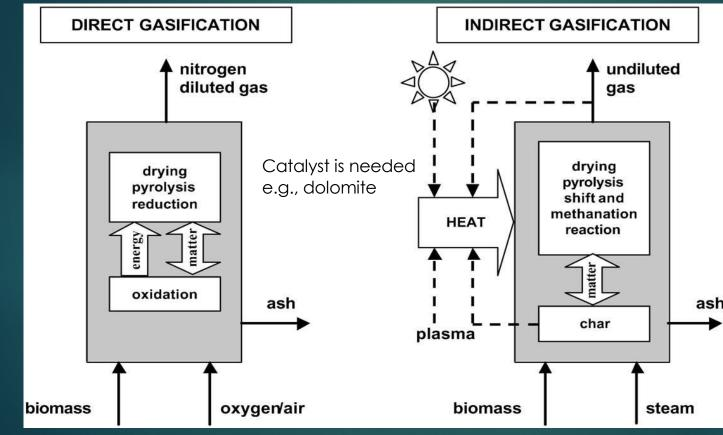
A chemical high temperature decomposition of organic matter into synthetic biogas (syngas), char and tar, and biofuel. It can convert one ton of MSW to more than 2 MWatt-h energy/ton of combustible MSW Modern future hydrogen based systems with indirect gasification can ash reach energy yield greater than 5 MWatth/ton of combustible sorted MSW
