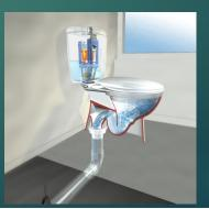
Dual flush toilet 3 and 6 liters/flush will save up to 75% of water for flushing when compared to standard pre 2000 toilet
