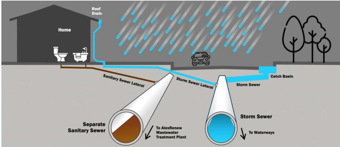
Separate Sanitary Sewer System
