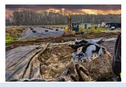
Through laboratory and field studies, smoldering-based thermal treatment was demonstrated to destroy per- and polyfluoroalkyl substances, the "forever chemicals" in soils. Of utmost importance to the DoD funding agency, ESTCP and SERDP, was understanding the mass balance of PFAS destruction.
